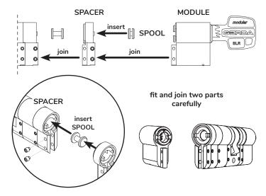
4 After you successfully combine the spacers, spools and modules, you should fix the cylinder with clamping screws using Allen key. Rotate the Allen key clockwise until it stops.
