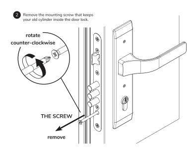
In order to remove the old cylinder you may need to insert and turn the key to hide the cam. Try to pull the cylinder gently with the key inside to find the right position when the cam is hidden inside the cylinder.
