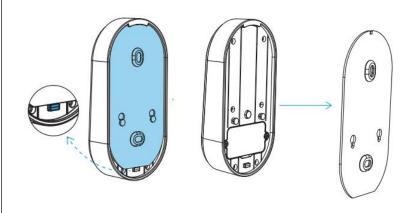
Press the button like the picture, and slide the panel.
